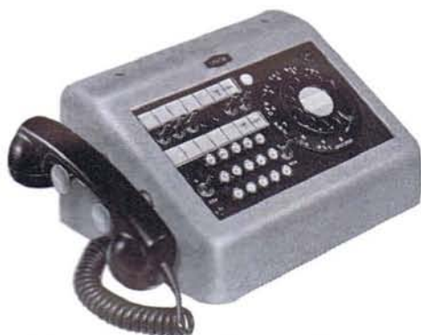
12-trunk turret for 40A and 88A units.
