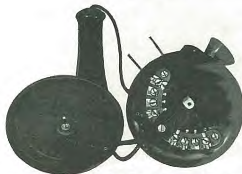
Fig. 9—Base Assembly of Standard Magneto Desk Set
