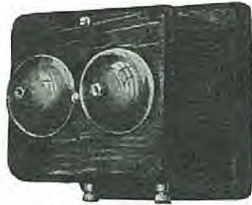
Fig. 12—Extension Ringers Are Mounted as Shown Herewith
