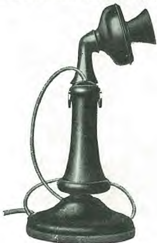
Fig. 7—Standard Local Battery Desk Set
