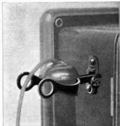
Fig. 1—Normal Position; receiver on the hook
