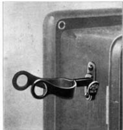
Fig. 2—Listening Position; receiver off and hook half way up
