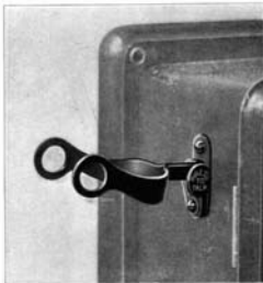
Fig. 4—Full operated position; hook up as far as it will go
