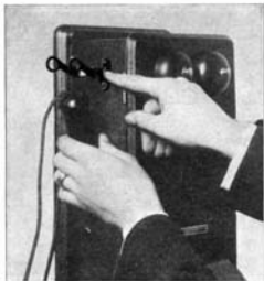
Fig. 3—Pressing button to put telephone in talking condition
