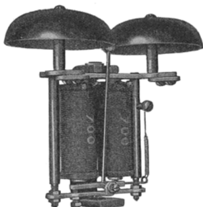
Illustrating General Design of Nos. 6 and 8 Type Ringers
