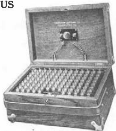
100 Cell Silver Chloride Testing Battery
