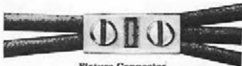
Fixture Connector Complete Connection Before Taping
