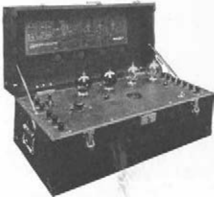
Vacuum Tube Amplifier used with No. 3-A Public Address System
