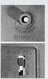
Some models have a three-position switch marked RING SEL on the bottom of the base. This switch may be set for one, three or five rings.
