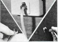
other end of the line cord into the base of The AutoMatic TelePhone. Some models will have the line cord jack at the back of the unit, and some will have the jack on the bottom of the base, as shown.
