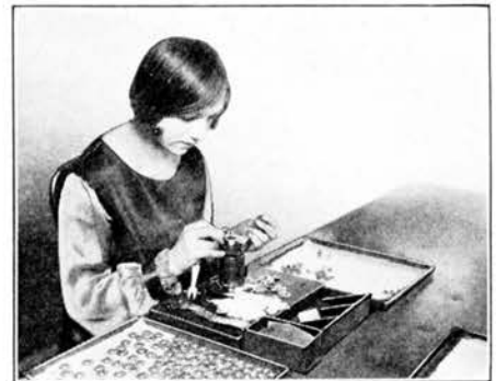
A round piece of mica forms one end of the carbon transmitter button of your desk stand type telephone instrument.
