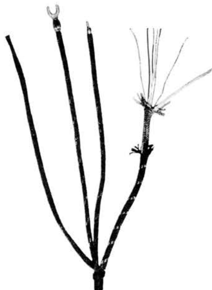
The cords which reach from your desk stand telephone instrument to the box on the wall or desk are covered with a silk braid to insulate and protect the wires. All telephones for use in tropical climates have connecting cords with silk insulations.
