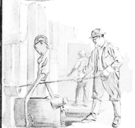
Open-hearth furnaces used in making aluminum alloys. Furnace in the foreground is being tapped.
