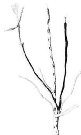
The flexible cords used to make electrical connections in telephone switchboards must be rugged and durable. The conductor strands are composed of thin copper ribbons, wound spirally in pairs around cotton threads, so that they will stand repeated bending without breaking. A group of these strands is next wound around a heavier cotton thread and is then wrapped with silk insulation. This unit is waterproofed and a cotton braiding is woven around it for protection and further insulation.
