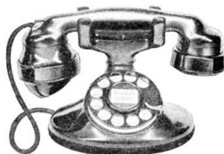
Copper is used in your telephone as wire and as an alloy in brass for plates and screws.
