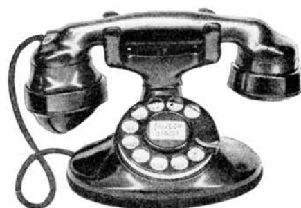
Alloy steel is used in the magnet and diaphragm of your handset telephone. The cradle and base are of zinc alloy; while the base plate, covered by leather, is of iron.
