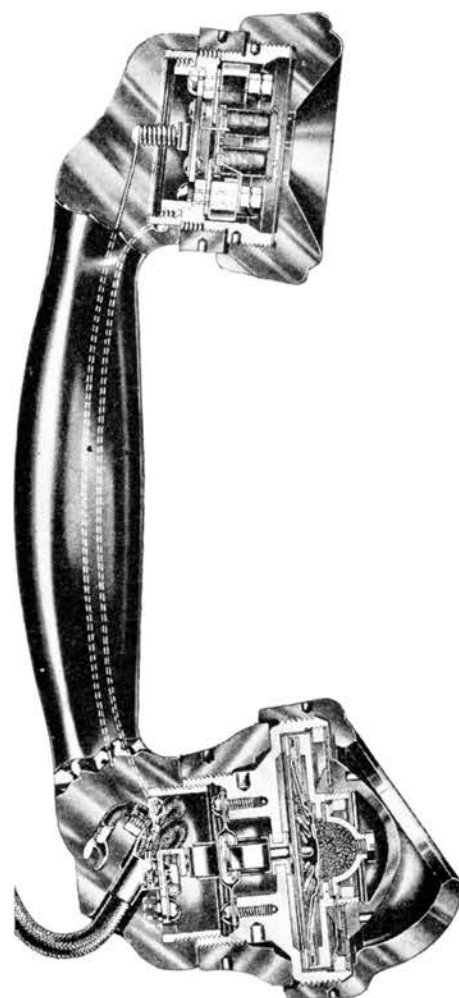
A cross section of your handset telephone. Practically all of the metal parts are made of various alloys that serve best each part for its particular job of giving telephone service. Some of the details of the transmitter and receiver are explained in later chapters.
