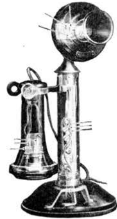
Nickel is sometimes used as a protective coating on the parts of the transmitter indicated by the three upper arrows and in the alloys used for connectors in the receiver and for springs in the body of the instrument.
