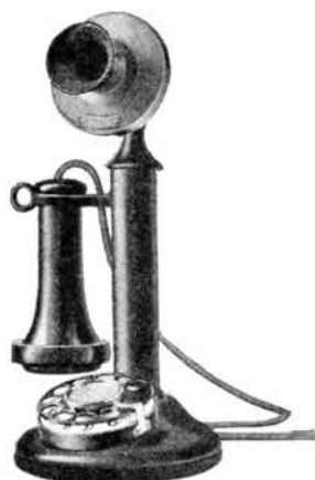
Alloy steel is used in the magnet and diaphragm of your deskstand receiver. The stem and base of this telephone are of brass, while the base plate (covered by felt) is of iron.
