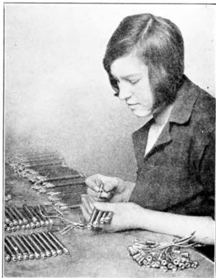
There is lead in the telephone fuse wires which protect the telephone circuits.
