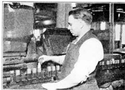
A condenser "potting" operation in which the condenser cans are filled with asphalt compound, and the units, composed of wound alternate layers of aluminum foil and paper, are inserted.
