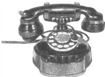
This is a hand set type of telephone having an applique base which contains the necessary keys.
