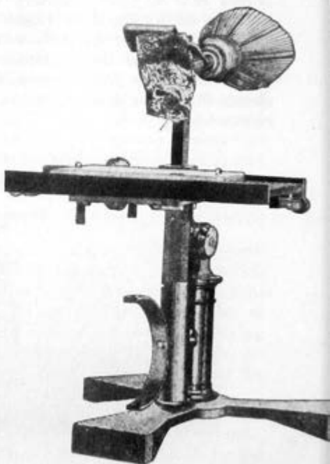
Fig. 1-2. Smoked-glass tracings of vowel sounds obtained from a phonautograph. Fig. 1-3. Bell's human-ear phonautograph with which he experimented in Brantford, Ontario, in 1874.
