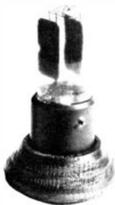
Fig. 4-40. Vacuum tube used in repeaters on the first transcontinental telephone line.
