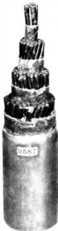
Fig. 4-11. Early cable with extruded lead sheath (1888).
