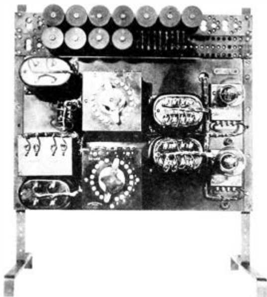
Fig. 4-48. Front view of Reading-type repeater. Equipment for one 2-wire circuit of loaded cable (22-type repeater circuit).
