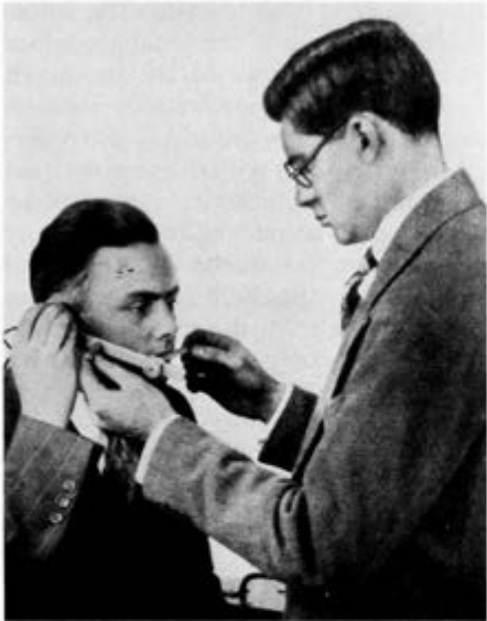
Fig. 3-62. A gauge being used for making head measurements to determine the proper dimensions of the handset. Fig. 3-63. Distribution of head measurement data. (Redrawn from Jones and Inglis 1932, Fig. 11)
