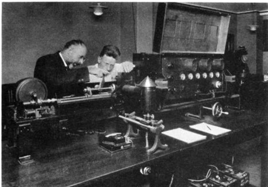
Fig. 7-30. Sending-end apparatus showing motor, film carriage, optical system, and amplifier-modulator. (Ives et al. 1925, Fig. 7)
