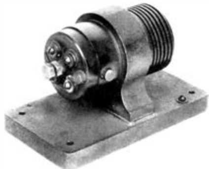
Fig. 4-34. The Shreeve mechanical amplifier (circa 1904). Fig. 4-35. The early Shreeve 1A repeater.
