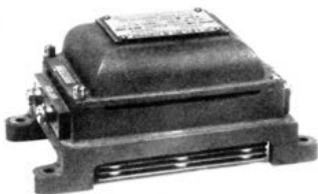
Fig. 4-34. The Shreeve mechanical amplifier (circa 1904). Fig. 4-35. The early Shreeve 1A repeater.
