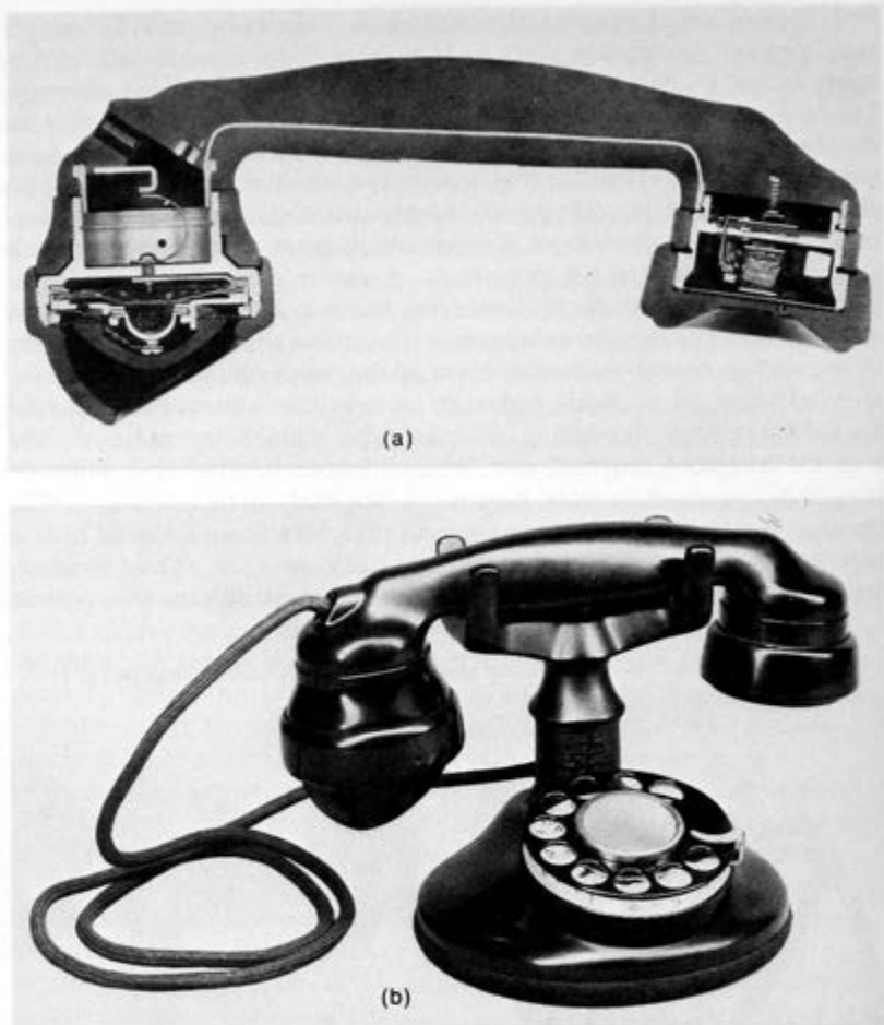
Fig. 3-68. (a) Cross section of early E1A handset (1926). (b) E1A handset and A1 handset mounting (1927).
