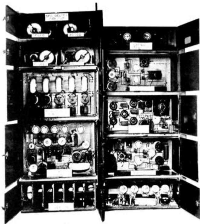
Fig. 4-58. Type A carrier telephone system—experimental equipment used in original carrier transmission tests at Maumee, Ohio, in 1917.
