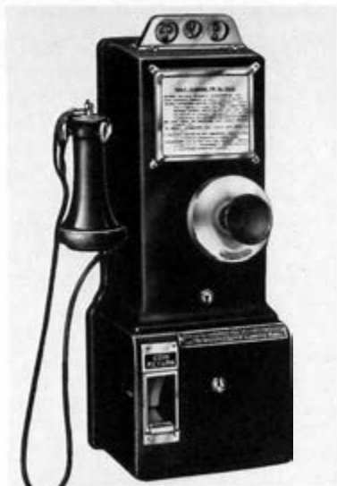
Fig. 3-72. Coin-operated telephone of the early 1900s with No. 7 collector. Fig. 3-73. Early No. 50A Gray/Western Electric coin box. (From Western Electric News of February 1916)
