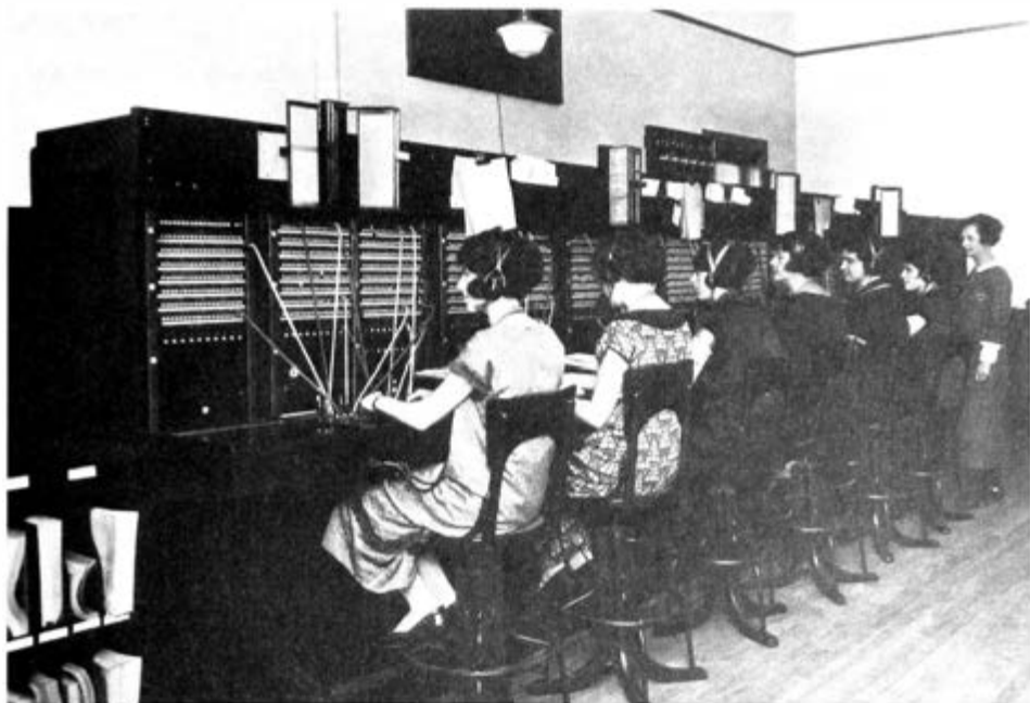
Fig. 6-107. A six-position No. 600C PBX switchboard, equipped with 480 station lines and 40 trunks, installed in Copley Plaza Hotel, Boston.
