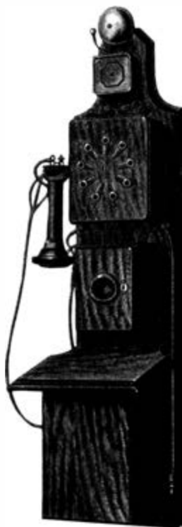
Fig. 6-93. Western Electric system for large buildings, telephone station set. (From Western Electrician , July 2, 1887)
