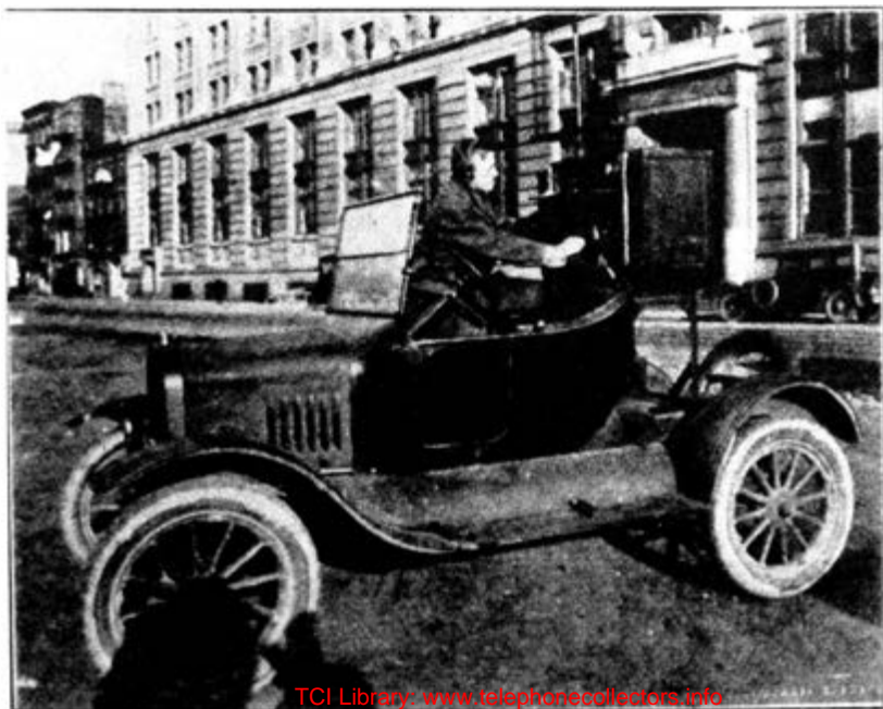
Fig. 5-65. Portable equipment mounted on a Ford roadster as used in 1925 broadcast survey. (Gillett, Proc. IRE , 1926, Fig. 2)
