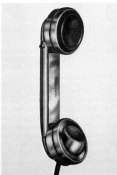
Fig. 3-57. Lineman's handset for use in common-battery system.
