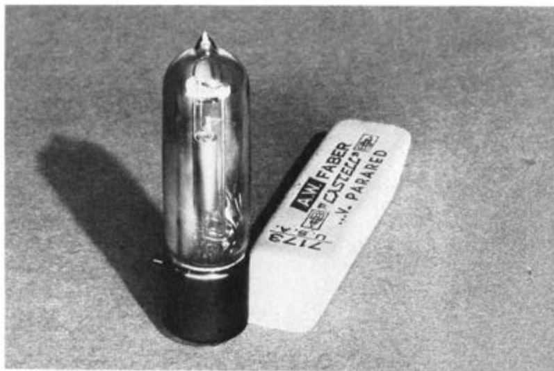
Fig. 8-26. The Peanut tube, patented by H. W. Weinhart.
