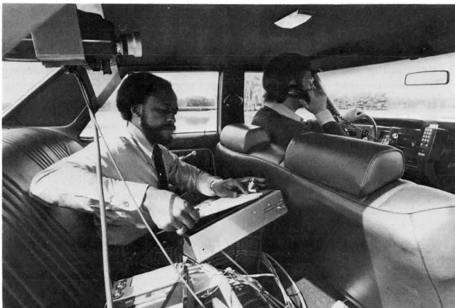
Figure 18-11. Human factors simulation. Laboratory and field simulations play a significant role in the design of user interfaces. Here, human factors engineers use a television camera to study the ease of placing and receiving calls while driving. Tests showed that placing a call with Advanced Mobile Phone Service telephones is as easy as tuning a car radio.
