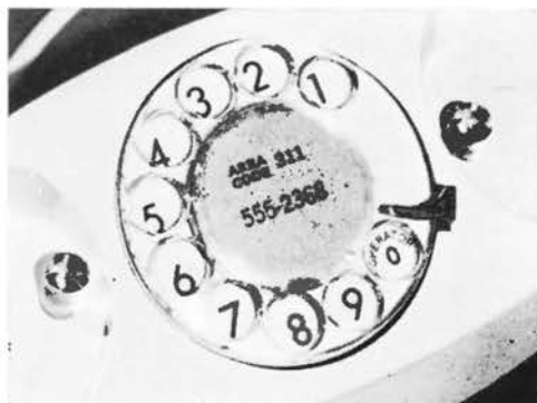
This model Princess phone designed for ANC shows but one number to a dial hole, this will cut down time needed to hunt letters.
