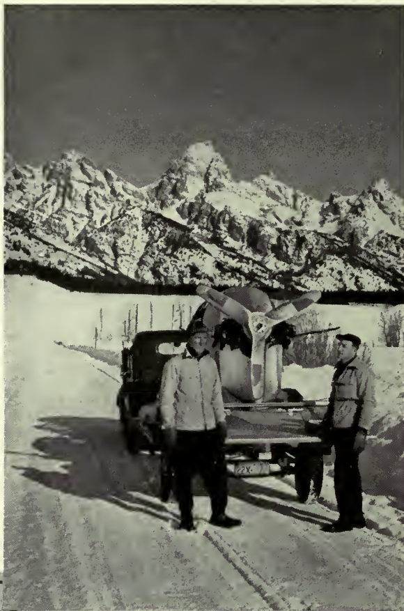
The ski-mounted sno-mobile on the trailer can carry two men over dry snow at 60 m.p.h. with their repair and testing equipment, emergency rations, snow shoes, and other winter necessities. It is part of the winter preparations of the Mountain States Telephone and Telegraph Company in Wyoming, whose Teton Mountains form the back drop for this picture
