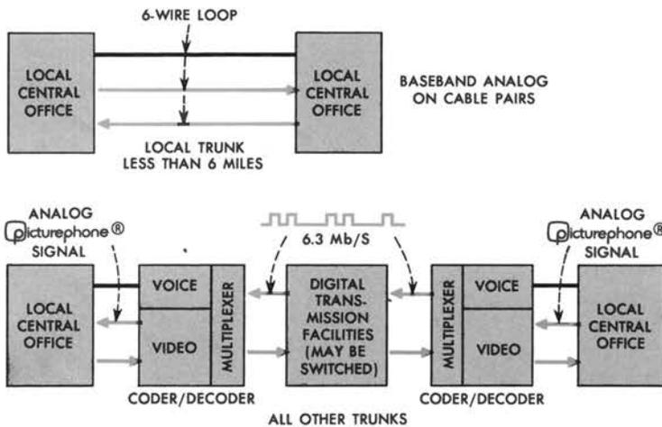
The Picturephone signal is transmitted between nearby central offices (less than six miles) in analog form (top). For transmission beyond six miles, the picture signal and the audio and signaling information are digitally encoded into a composite 6.3-Mb/s signal and decoded again at the distant office.
