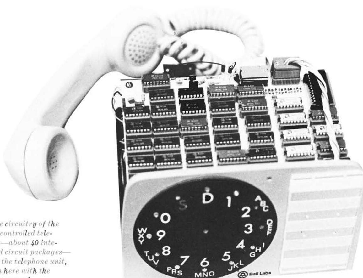
*All the circuitry of the voice-controlled telephone—about 40 integrated circuit packages—fits in the telephone unit, shown here with the cover removed.*
