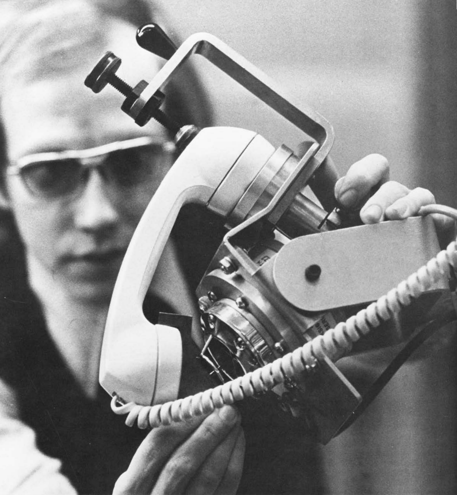
At Bell Laboratories' Indianapolis location, Dennis Burcher of the Telephone Circuits group prepares to make acoustic measurements of the new G36 telephone handset.
