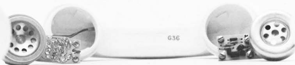
Built into the G36 handset are two solid-state gain units: one for transmit (left), one for receive (right).
