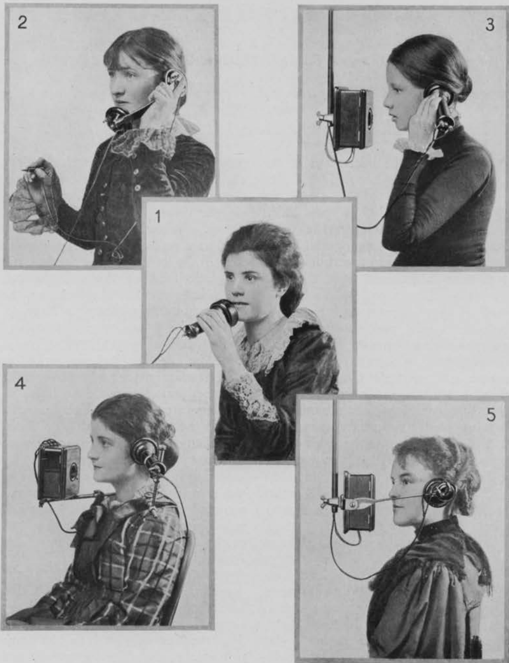
1, Bell's hand telephone in use as a transmitter. The same instrument acts as a receiver with incoming voice-currents; 2, Transmitter and receiver were mounted at opposite ends of a bar magnet in this operator's handset of 1879; 3, An early Blake transmitter and associated receiver, mounted to leave one of the operator's hands free; 4, Instruments the same as those of Figure 3, supported in a "Gilliland harness" to free both hands; 5, Another mounting arrangement keeping both hands free
