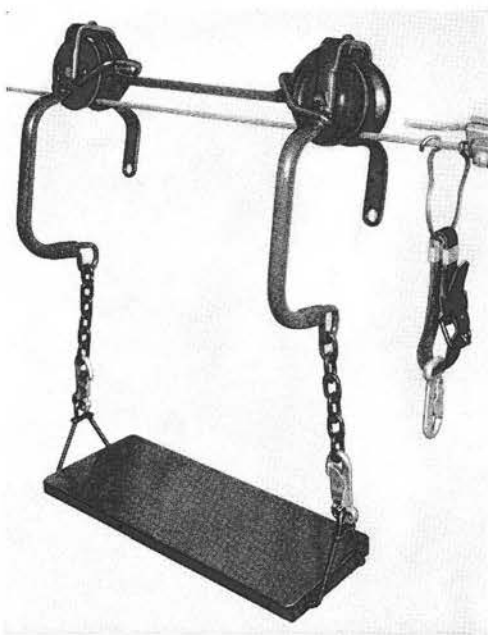
Fig. 4—The construction and maintenance of aerial cable frequently requires that workmen ride a cable car
