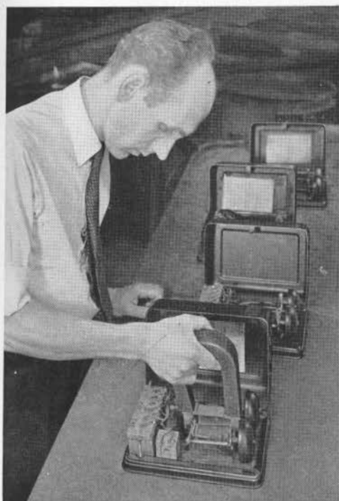
Fig. 1—The remagnetizer can be used on ringers assembled in the subscriber sets housed in metal and phenol plastic boxes
