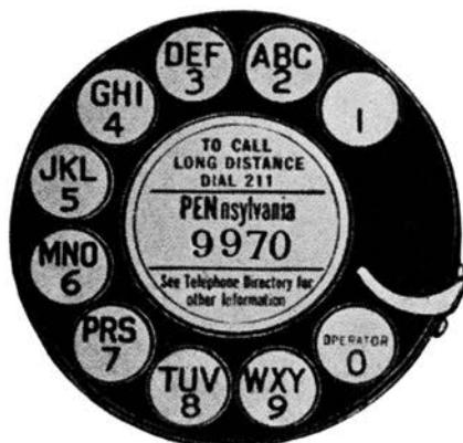
Fig. 2.—A dial that came into use in the Bell System as a result of Blauvelt's invention.
