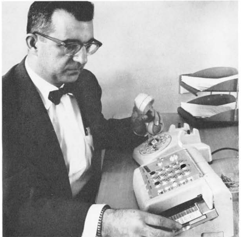
Western Electric Co. engineer prepares to send business items through the compact card reader of the new Dataphone system.
