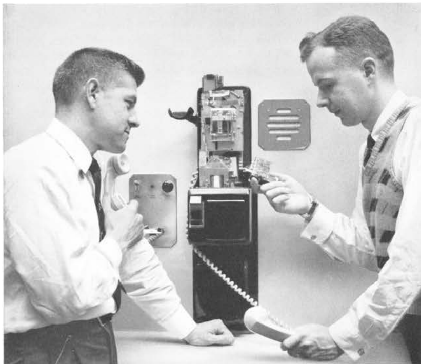
This arrangement demonstrates how trial models of new coin-telephone work. The author, left, holds handset that is comparable to operator's headset, and L. A. Strommen holds new coin-signal network in his right hand.
