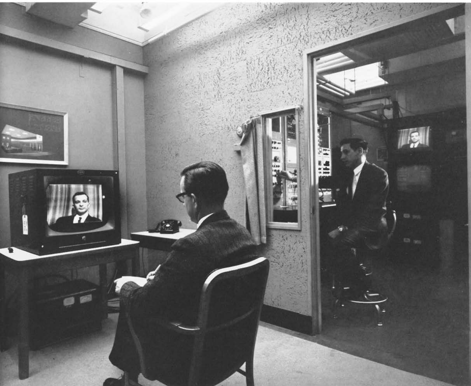
The variable-parameter television system laboratory. R. H. Rosasco, at the control panel, adjusts picture parameters which the author, A. D. Hall, in the viewing room, judges them according to standards of clarity, brightness, etc.
