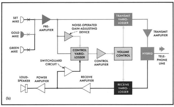
When the PCT is in the receive mode, upper diagram (a), incoming speech is tapped off by the switchguard circuit. The control variolosser and control amplifier then increase the loss in the transmit variolosser, almost cutting off the trans-
