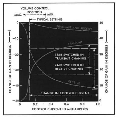
The PCT's transmit and receive variolossers operate together—when one increases its loss, the other reduces its loss. The control current for each variolosser ranges between 1.0 milliampere and a lower current, determined by the setting of the volume control. In the receive mode, the current is set by the volume control. When the user speaks, the current increases, raising the loss in the receive channel and decreasing loss in the transmit channel.
