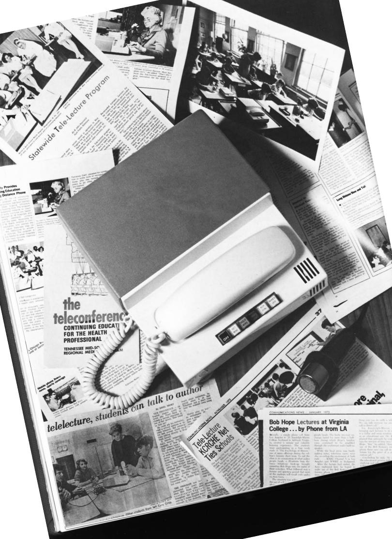
The Portable Conference Telephone (PCT) allows voice communications among groups in widely separated locations. With extension microphones and with more power than its sister unit, the speakerphone, the PCT can be used for large classes or conferences.
