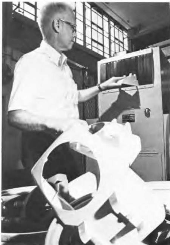
**Turning scrap into scraps.** Herb Kern of the Plastics Research and Development department feeds battered plastic telephone housings into a knife-blade granulator.
