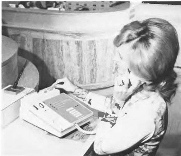
Account balance. Customers of Central Trust Company in Cincinnati use Transaction telephones to check the balance in their checking and savings accounts. Here, Carolyn Chitwood of Cincinnati Bell runs her bank card through the card reader and keys in her personal code. She will soon hear the balance over the audio response system. An advantage of the audio response is that only the customer can hear a balance, whereas anyone nearby could see a visual display.
