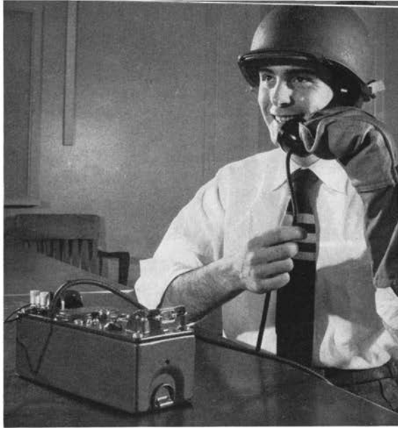
In the new telephone set, the handset is shaved at the ear-piece end so it can fit comfortably beneath a battle helmet, and the “press-to-talk” switch can be operated when wearing Arctic mitts. Tony Prestigiacomo posed the picture.
