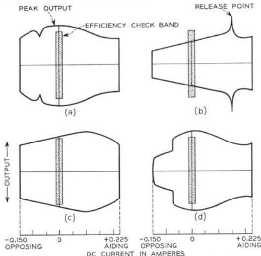
Fig. 9—Oscilloscope traces reveal mechanical flaws. A—Burr or dirt on diaphragm seat. B—Ground separation too small. C—Weak magnet. D—Obstruction in auxiliary air-gap.
