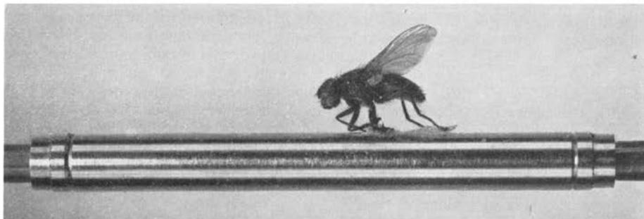
*Comparison of the transistor repeater with an ordinary house fly —  $3\frac{1}{2}$  times actual size.*
