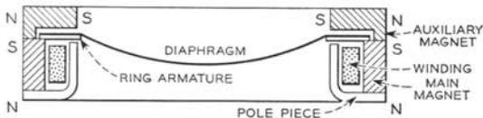
Fig. 3—Simplified view of ring armature receiver.
