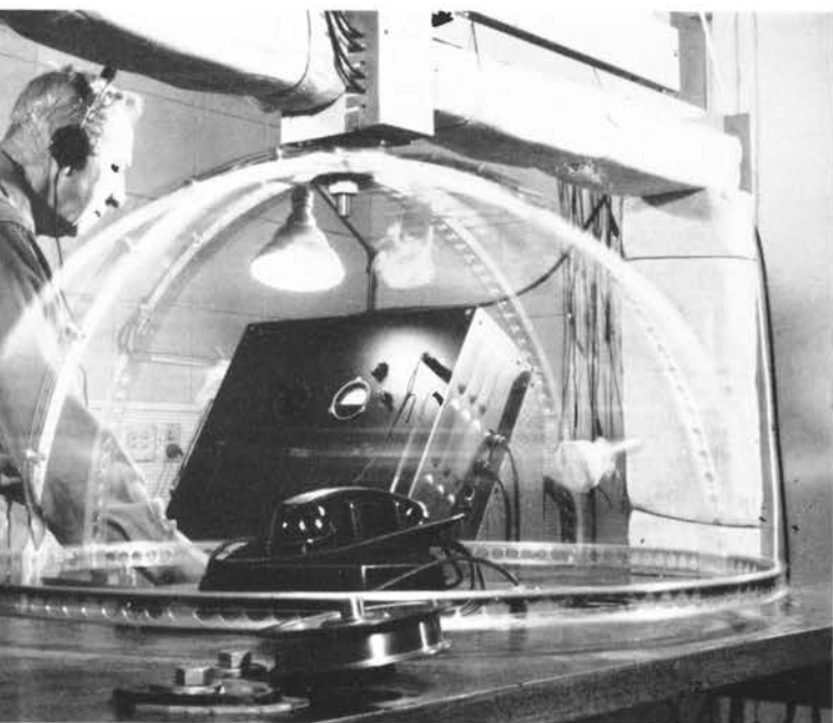
Fig. 6—The author determining sound spectrum of ringer with sound integrator and frequency analyzer.
