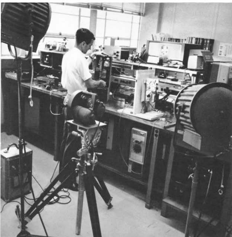
C. D. Hays works with a laboratory model of the 1A1 Coin Telephone. Movie camera gives a high speed series of pictures showing various points in a coin's traverse down the telephone chute.
