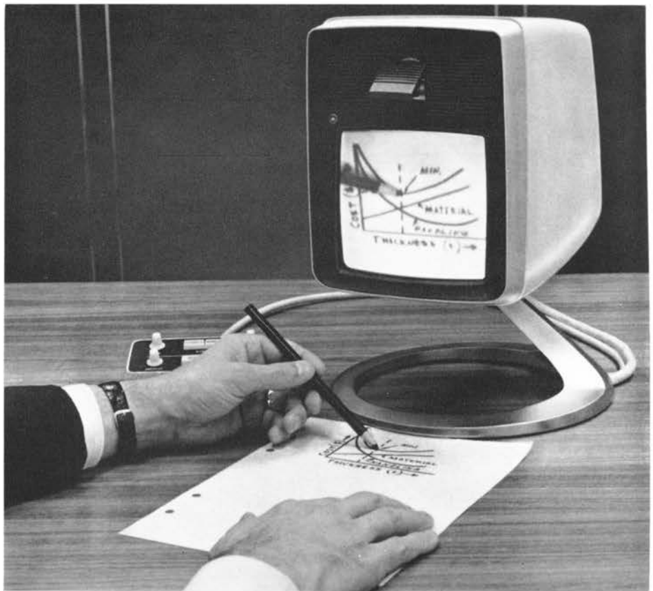
The Bell System's new Model II PICTUREPHONE set can be used to transmit drawings or charts by setting the camera focus at one foot. In the photograph, the "self-view" option is being used to position the graph while it is transmitted.
