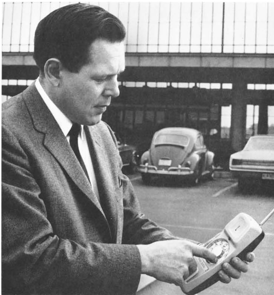
C. E. Paul dials a number on an experimental lineless telephone. The unit, which provides simultaneous two-way conversation, connects with the telephone network via a radio link to a fixed station connection to a telephone or extension line.
