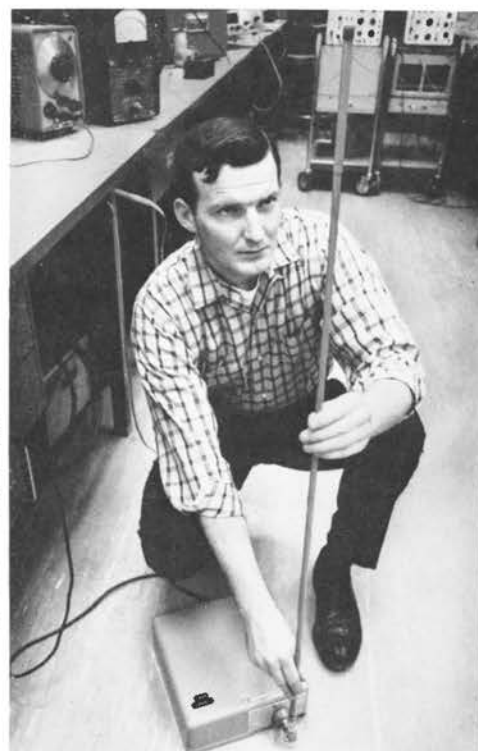
C. E. Paul dials a number on an experimental lineless telephone. The unit, which provides simultaneous two-way conversation, connects with the telephone network via a radio link to a fixed station connection to a telephone or extension line.
