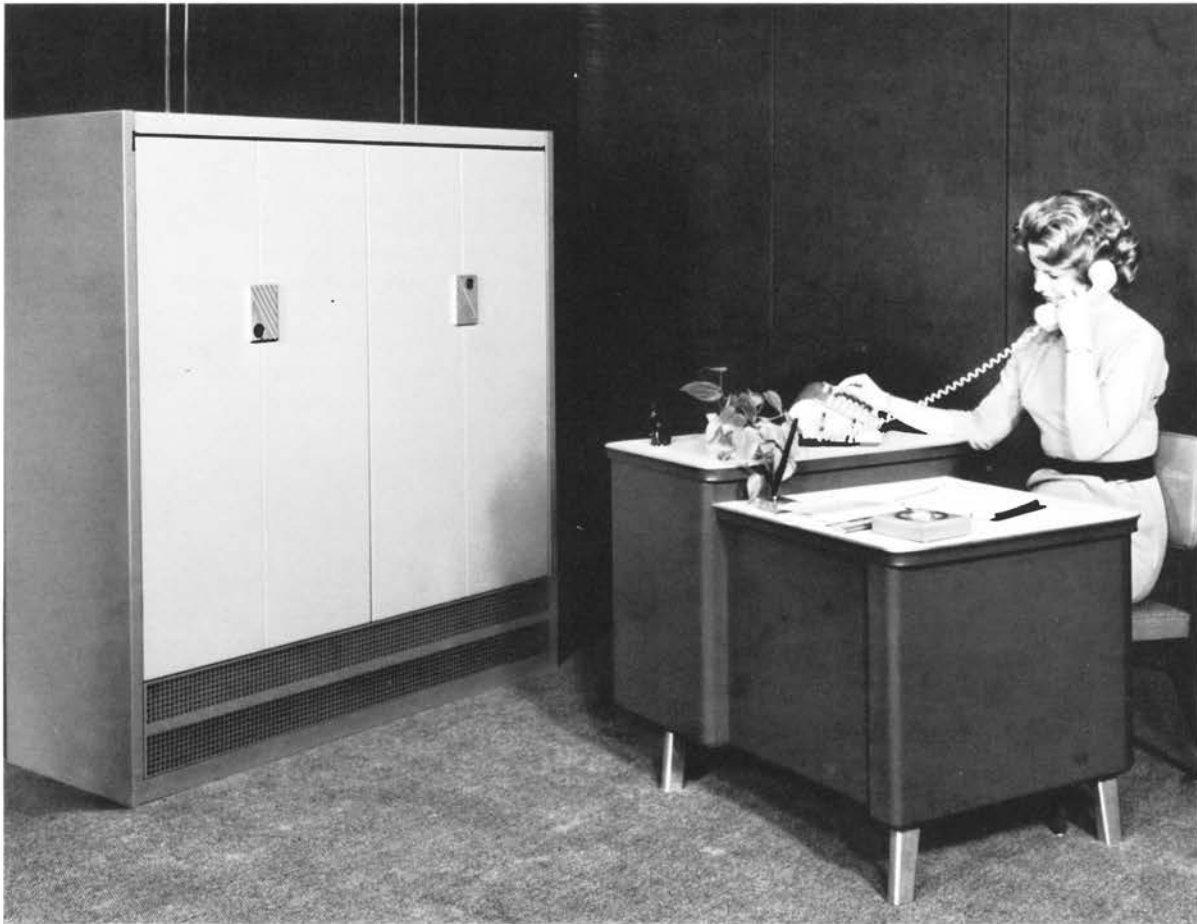
The switch unit of the No. 101 ESS is installed on the customer's premises, while the control unit is located in a central office. The switch unit cabinets are designed to blend with modern office decor.
