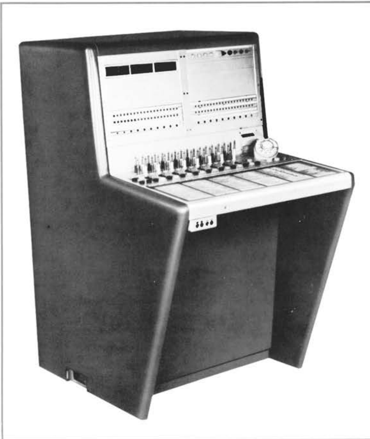
A cord-type, multiple switchboard, the 608A presents a new, modern appearance, occupies less space than earlier models, and has additional service features. The board was first introduced in the late 1950's and still remains as a popular standard today.
