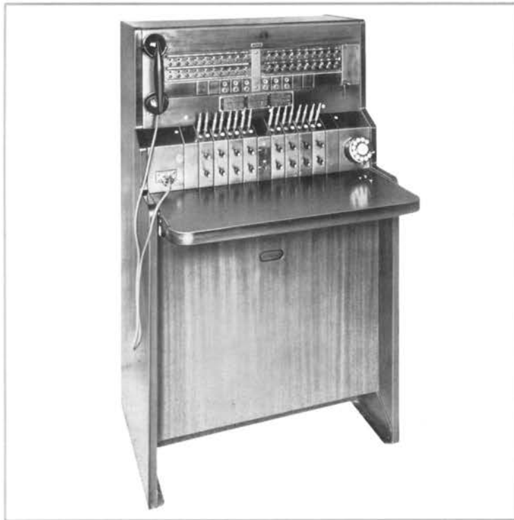
The 555 PBX, developed after World War II, was the first system to use the efficiency of plug-in units for many circuits.
