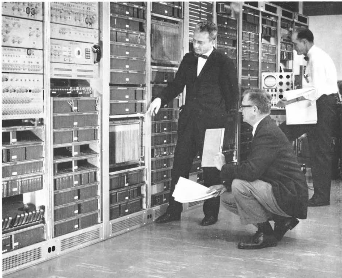
M. A. Townsend (standing) and W. F. Means inspect one of the twistor memory stores in an experimental control unit of the No. 101 ESS at Bell Laboratories. Mr. Means holds a program card. H. F. Priebe, in background, checks equipment in the line data frame portion of the unit.
