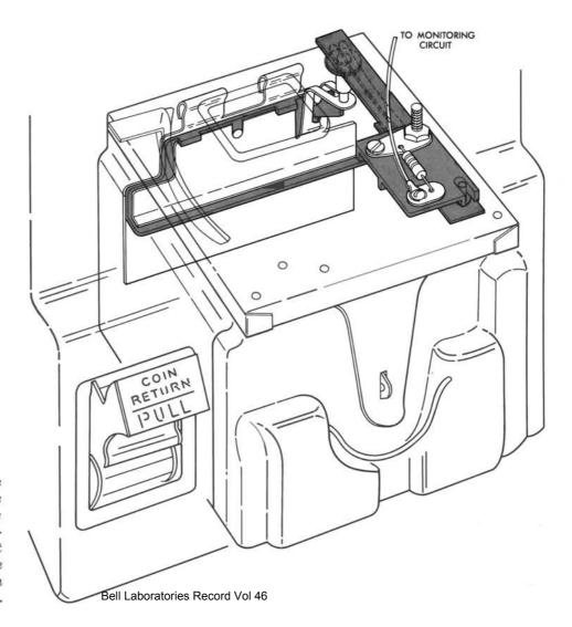
The coin level sensor clips into place inside the coin receptacle. When the receptacle is 68 percent full, the coins contact the sensor, sending an electrical indication through the contact stud in the receptacle cover to the terminal board mounted separately in the base of the telephone housing.
