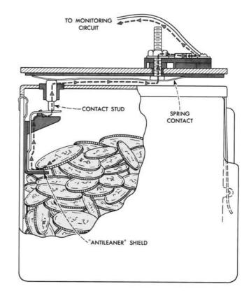
The lower edge of the signal strip is turned outward to provide a horizontal ledge for the coins to rest upon. This assures reliable contact forces between the coins and the sensor and reduces the probability of signal instability caused by coins being jarred out of contact with the sensor by subsequent deposits. A plastic "antileaner" shield extends out from beneath the ledge to prevent premature triggering by coins falling on edge and leaning against the sensor.
