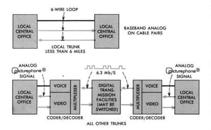
The Picturephone signal is transmitted between nearby central offices (less than six miles) in analog form (top). For transmission beyond six miles, the picture signal and the audio and signaling information are digitally encoded into a composite 6.3-Mb/s signal and decoded again at the distant office.
