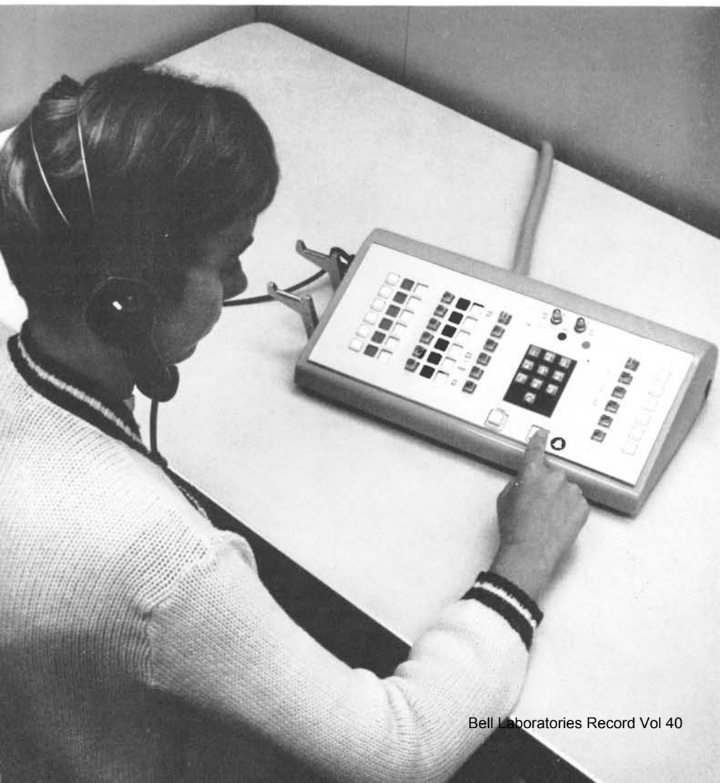
New compact console designed for PBXs served by CENTREX. It can be conveniently placed on a desk top and used by an attendant, or by a company receptionist.
