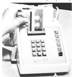
New plastic cards, the size of standard credit cards, and card dialer telephones have been designed by engineers at Bell Laboratories in Indianapolis. The cards can be used to dial telephone numbers automatically or transmit information over the telephone system to computers.
