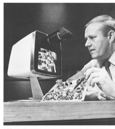
A "C-mount" set with a zoom lens transmits a detail of a printed-circuit board. The zoom lens can be conveniently adjusted for different fields of view. There is no necessity for changing lenses.
