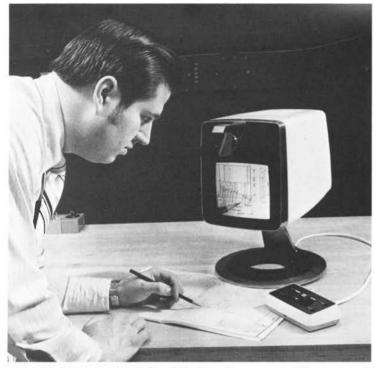
When the Picturephone<sup>®</sup> set is placed on a specially designed rolling base, it can be moved around to view details on a large drawing. A zoom lens allows the user to adjust the magnification.
