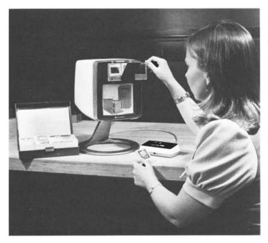
A clear plastic holder and a close-up lens allow the viewer to send images of 35-millimeter slides. A reflector at an angle throws ceiling light on the slide—additional light is not needed.
