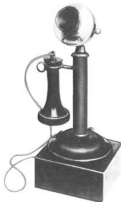
Portable telephone of 1904 (above) was designed for restaurants, with the pedestal design—forerunner of the 1919 "candlestick"—but with speech-circuit components in the base. At right is the first public coin phone of 1889.
