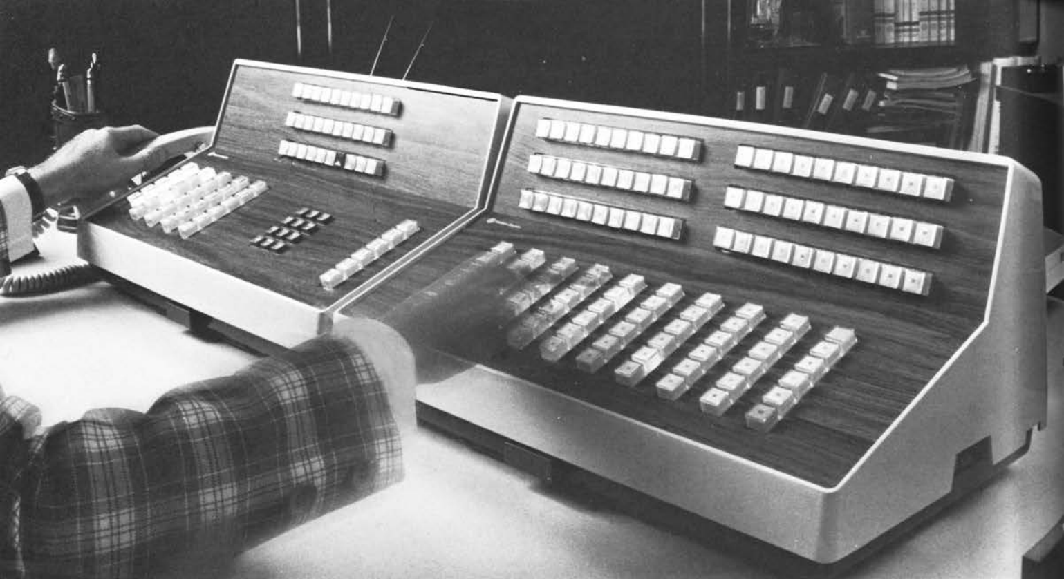
Big system. This large Com Key 2152 system is equipped with a 21-line attendant console at the left, and a direct-
