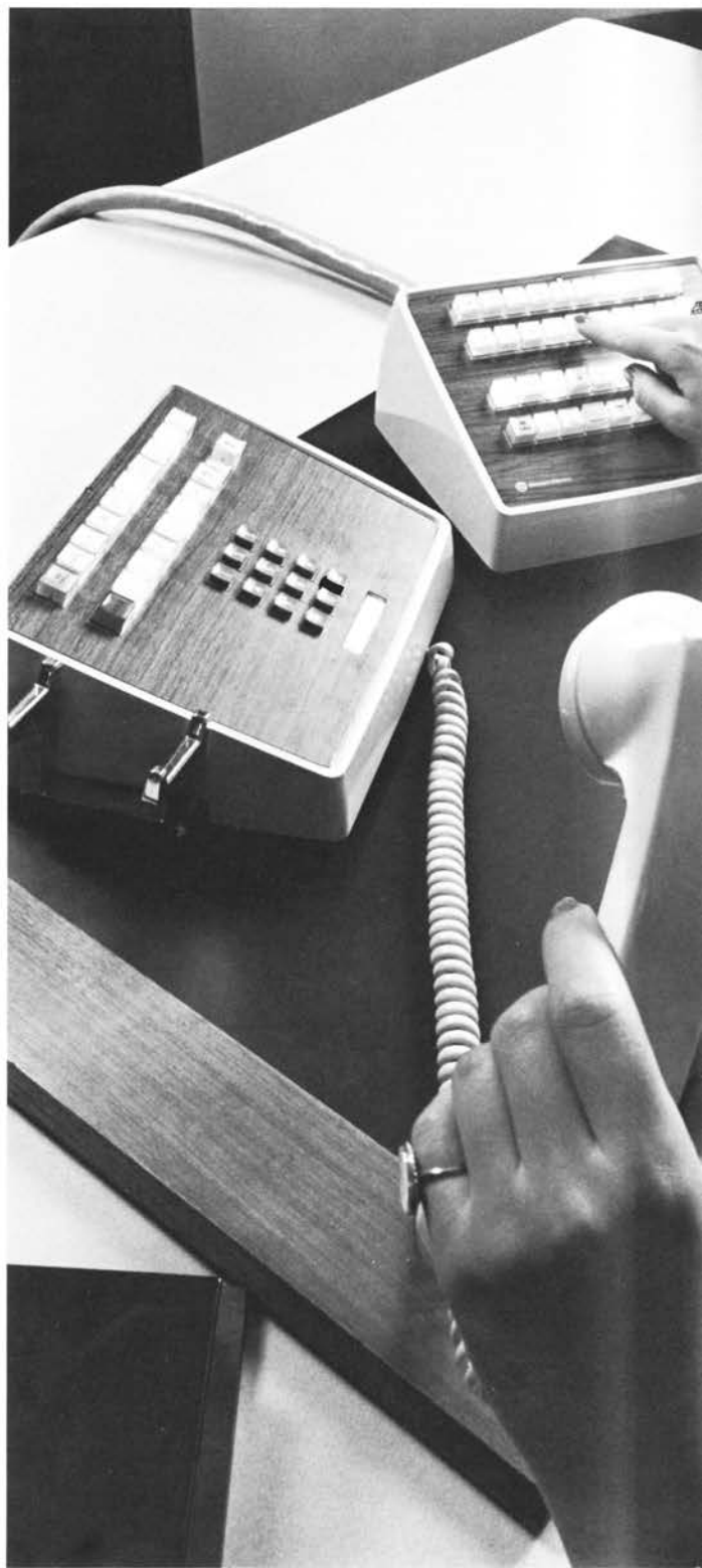
Medium-size system. The larger Com Key 1434 system has additional buttons for up to 14 lines, as well as 34 direct-station-selection codes.
