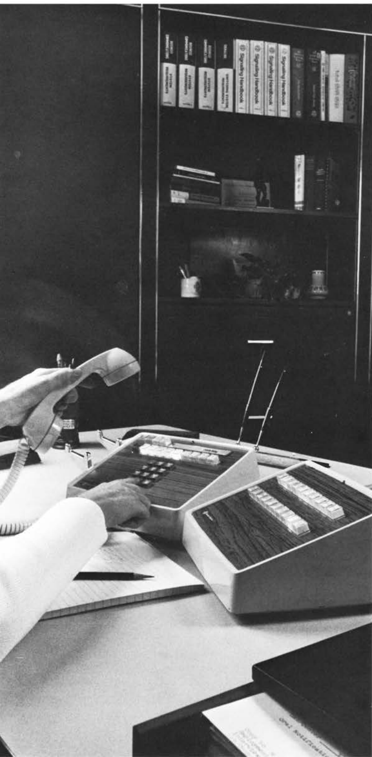
Small system. The Com Key 718 system has 7 lines and 18 phones. At the right is the optional direct-station-selection console with station-busy indication.
