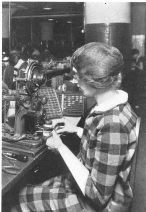
Miss Juliette Charpin manipulates the electric welding of the grid
