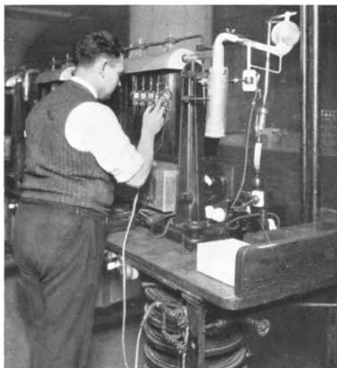
After completing the exhaust of a tube, B.J. McNally seals it off the pumping manifold
