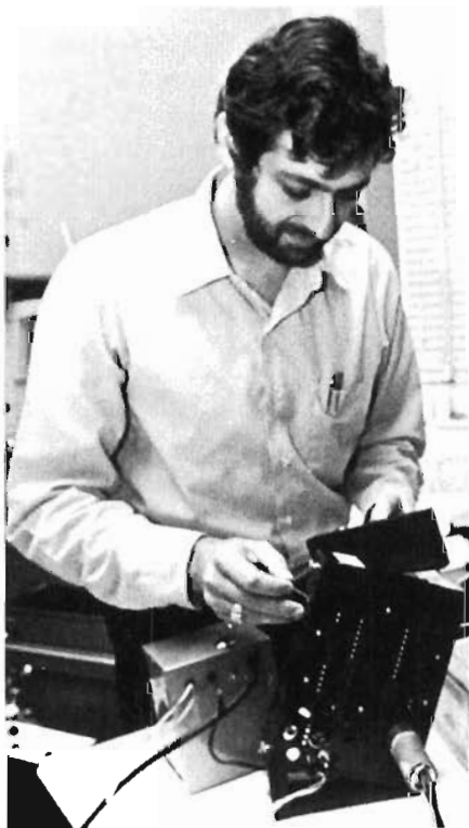
Fig. 6-17. A. A. Lamola operating the original hematofluorometer used to detect lead poisoning by examination of a drop of blood.
