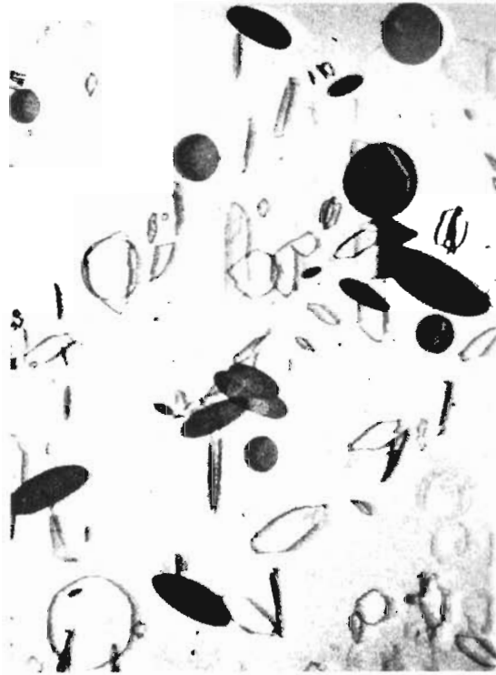
Fig. 19-13. Stacking faults in silicon that result from oxygen precipitation shown by X-ray topography.
