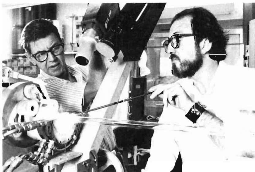
Fig. 13-2. J. B. MacChesney (left) and P. B. O'Connor, co-inventors of the MCVD technique in the process of making low-loss optical fibers. The silica tube and its contents are heated until they collapse into a solid glass rod, from which about 10 miles of fiber can be drawn.
