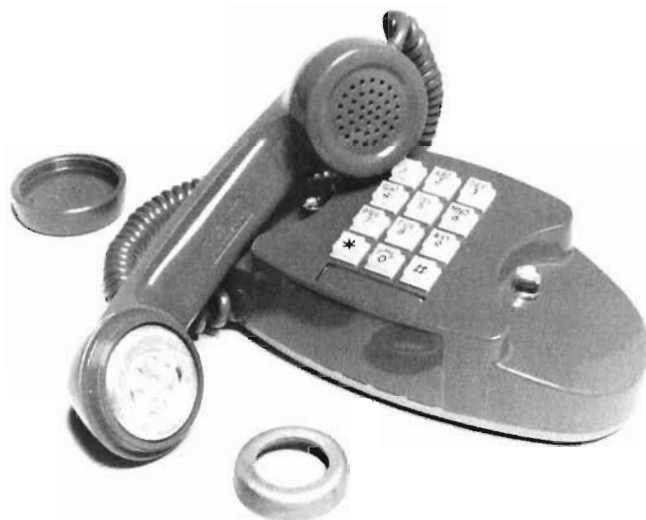
Fig. 12-9. Ring-shaped, Chromindur permanent magnet (bottom) used in the U-3 telephone receiver.
