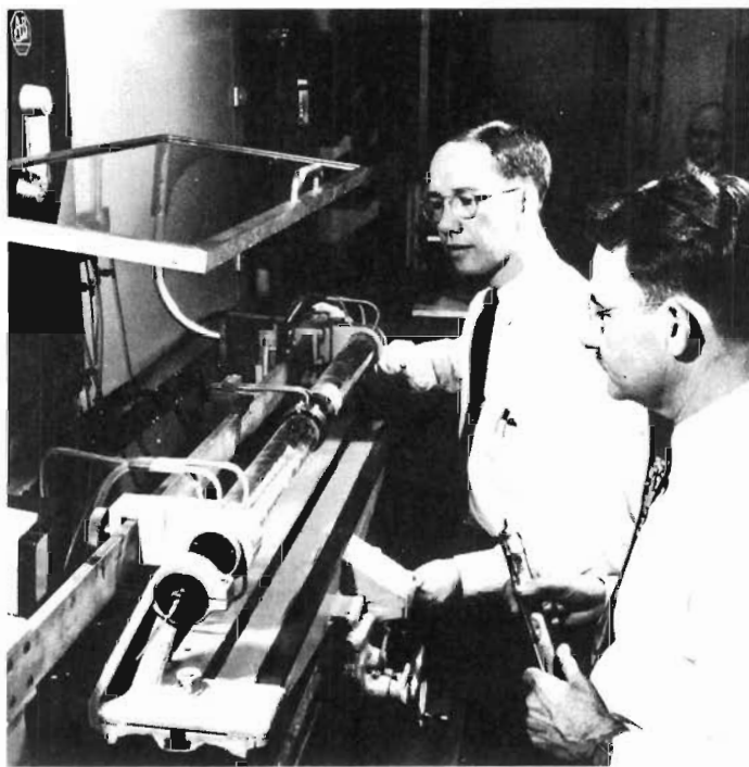
Fig. 11-4. W. G. Pfann, inventor of zone refining, shows the first zone-refined single crystal of germanium to J. H. Scaff, who pioneered in the growth of germanium and silicon ingots of either p-type or n-type conductivity.
