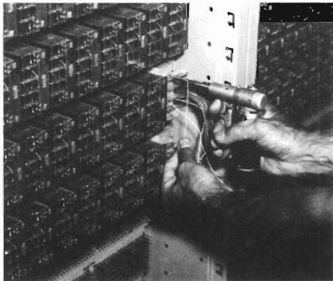
Fig. 5-23. Wire-wrapping gun used to achieve solderless electrical connections to apparatus terminals.
