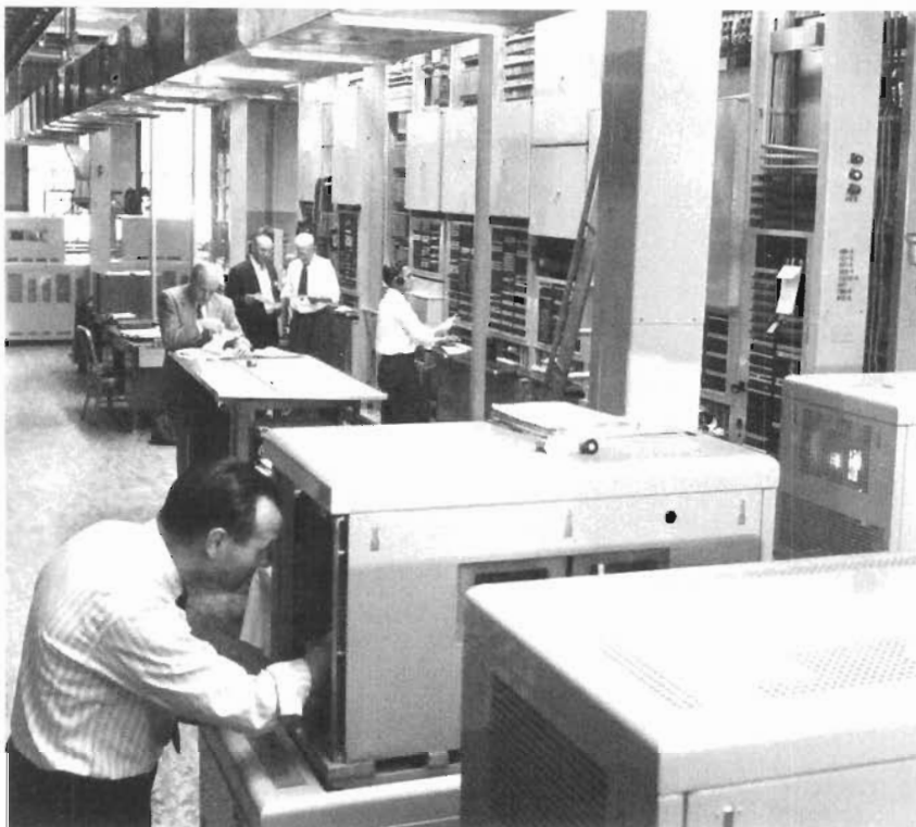
Laboratory installation of card translators, about 1952. A key system element in the growth of nationwide dialing by customers, the card translator interpreted the six digits of the area code and office code of a called telephone number. These digits caused one metal card to drop down from a stack of about 1000 cards. According to which holes holes in the cards were or were not enlarged, light passed through to photo-detectors to specify the information needed to select a route for a long distance call.
