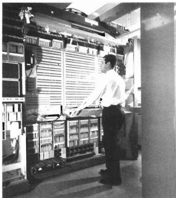
Fig. 9-44. R. S. Cooper using the No. 1 ESS program test console, which displayed the execution of the ESS program and aided debugging.
