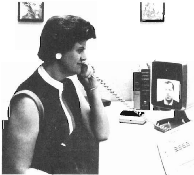
Fig. 13-47. Attendant arrangements for PICTUREPHONE service. All procedures were the same as those for telephone PBX service, or natural extensions of these procedures.
