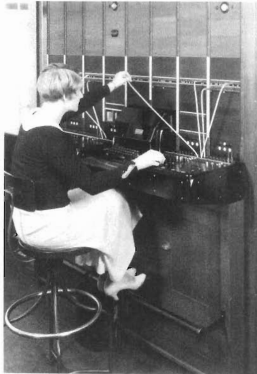
Fig. 13-84. Manual switchboard adapted to teletypewriter service, 1931. Instead of a telephone headset and microphone, the operator used the teletypewriter keyboard.
