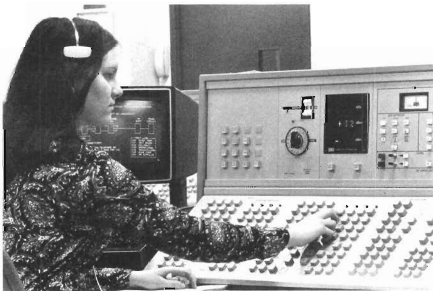
Fig. 12-7. Barbara Reed, Long Lines, at a 51A test position of the circuit maintenance system 1A, which gives craftspeople access to No. 4 ESS data bases and circuits for trunk maintenance.
