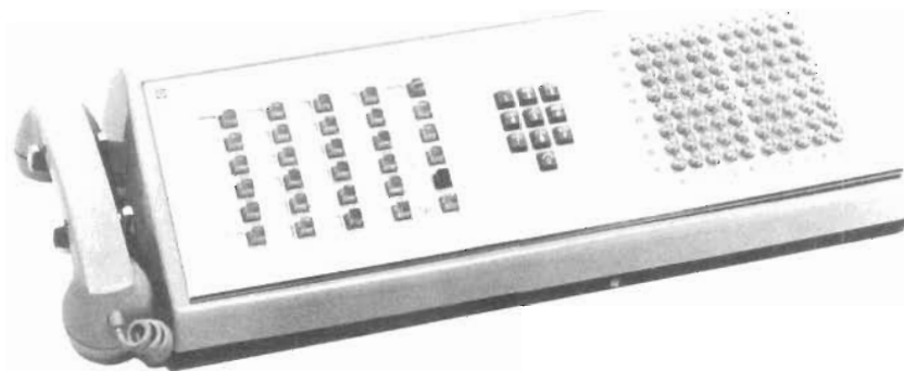
Fig. 13-25. Attendant console for the 800A PBX. Operation was simplified by using different flashing rates of a single lamp to indicate various supervisory states. ( Communications Présentées au Colloque International de Commutation Electronique , Paris, March-April 1966.)
