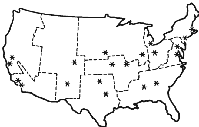
Fig. 12-11. Plan of signal transfer points for common-channel interoffice signaling. Call information transmitted over CCIS offers potential for many new services. ( IEEE Symposium Record, International Switching Symposium, Kyoto, Japan, October 1976. )
