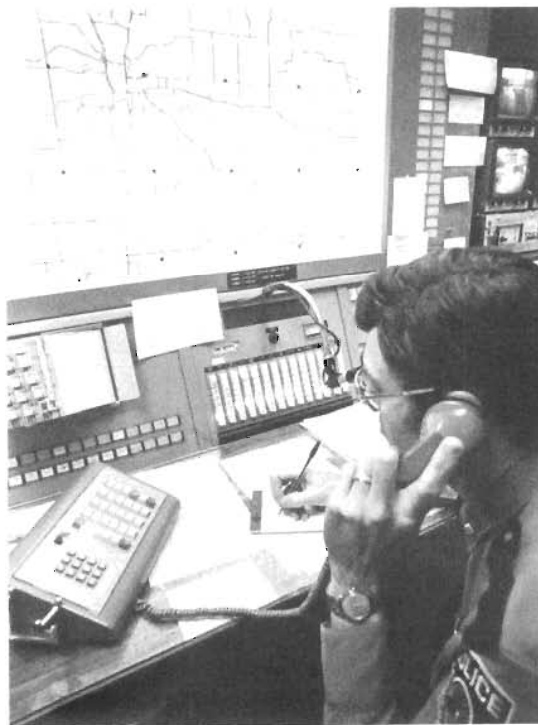
Fig. 11-14. A 911 emergency position. Special provisions are made to call back the caller and to force the release of emergency call connections.
