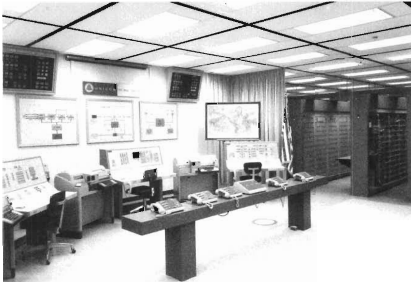
Fig. 9-46. Part of the UNICOM test model—switching center consoles and digital and analog station control sets.
