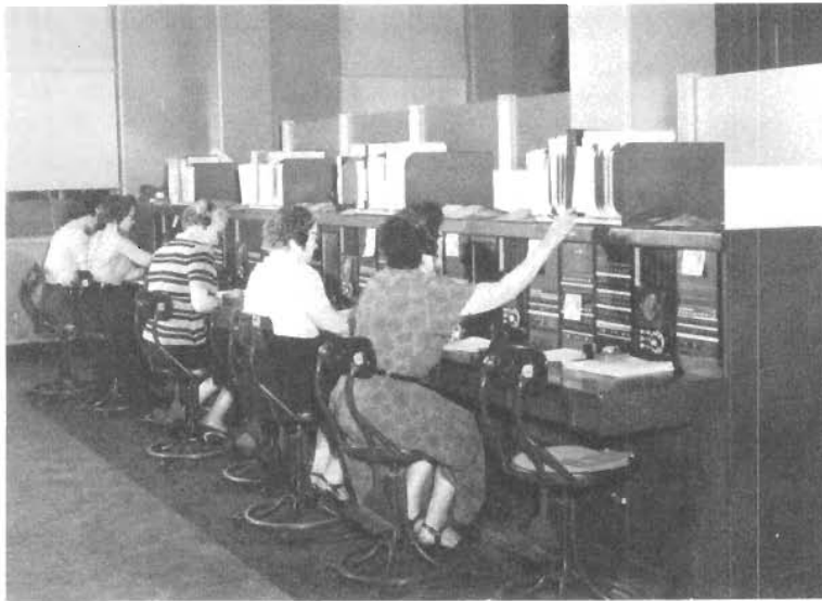
Fig. 11-18. New York City installation of No. 12 service observing desks, developed in 1949 to centralize this function for various central office systems and switchboards.
