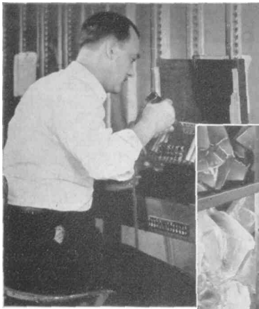
Quartz crystals from Brazil are carefully selected for use in telephone filters and radio oscillators.
