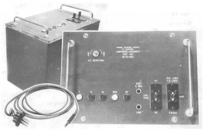
Fig. 1. Views of Linefinder Continuity Test Set To Show Location of the Lamps, Jacks, Keys and Dial Tone Detection Potentiometer. The Test Cord is Also Shown.
