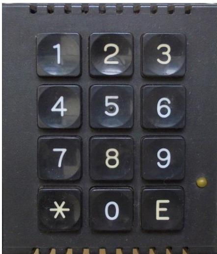
This is the keypad of the "Apart 2001;" it is of the GDR standard dial-pulse type, but its operation is slightly different: the "star" key is dead (there is no redial function), and the "E" key is an "earth" or "ground" key.
