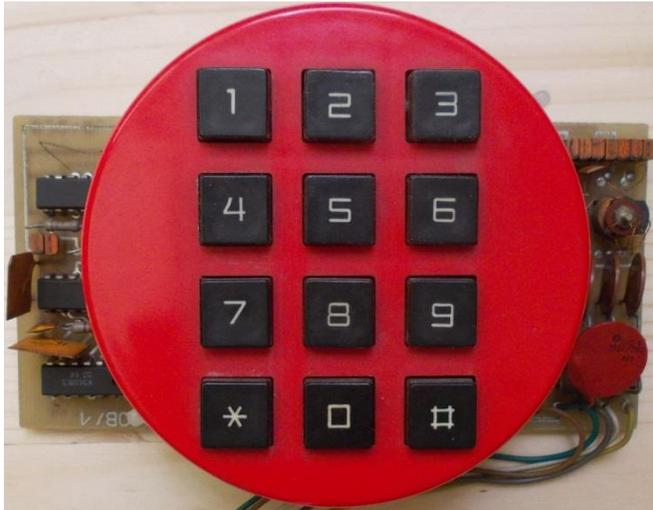
This was the GDRs first attempt at a telephone keypad (from the early 1980s), based on a 40 pin soviet microcontroller ... **it is believed that this keypad was only produced in small numbers and was intended to be the prototype for following keypads.**
