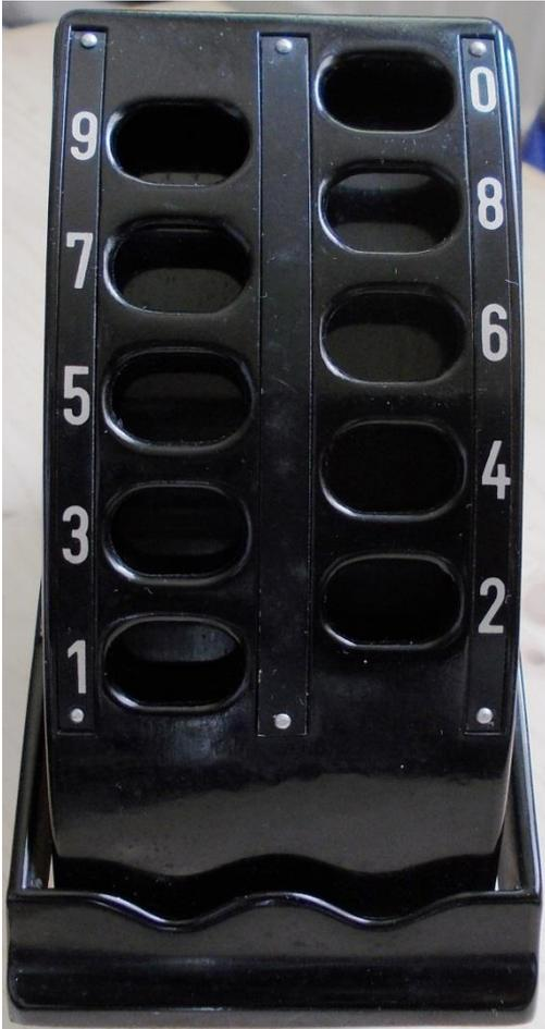
As can be seen, the non-movable portion of the drum no longer carries the digits, which are now on strips of electrically oxidized aluminum, riveted along the outside edges of the finger-hole arc.
