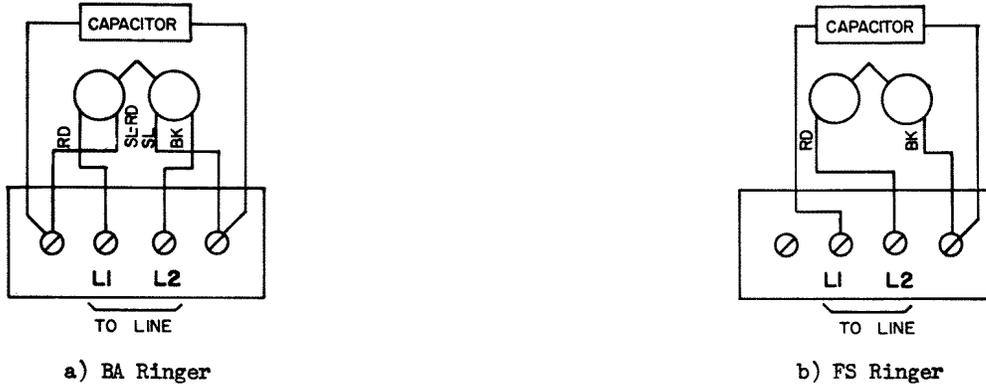
Fig. 2 WIRING DIAGRAMS
