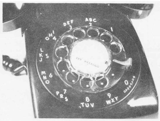
Fig. 3-3 REPLACING LUCITE FINGER PLATE
