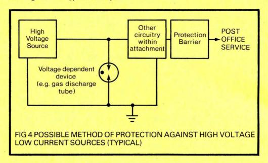
c. Voltage dependent device(s) may be fitted to conductors connected to the Post Office service. The voltage dependent device(s) may be part of a fuse disconnection barrier. A typical arrangement is shown below in Figure 5:
