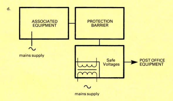
Both the supply transformer shown and the protection barrier must meet Post Office protection requirements; see 5.2. The protection barrier may be any of the types listed in b. above.
