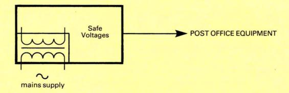
The supply transformer(s) must meet Post Office requirements (see 5.2.2). If there is associated equipment that is separately powered, this must either meet Post Office protection requirements or must be isolated by means of a protection barrier. (See c. and d. below).
