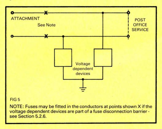
The voltage dependent device(s) must meet the following requirements:
