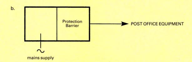
The protection barrier must meet Post Office protection requirements and may be any of the following types:
