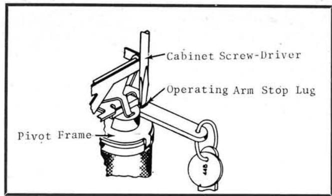
Fig. 8 Using gauge and screw-driver to check and adjust armature operating travel.
