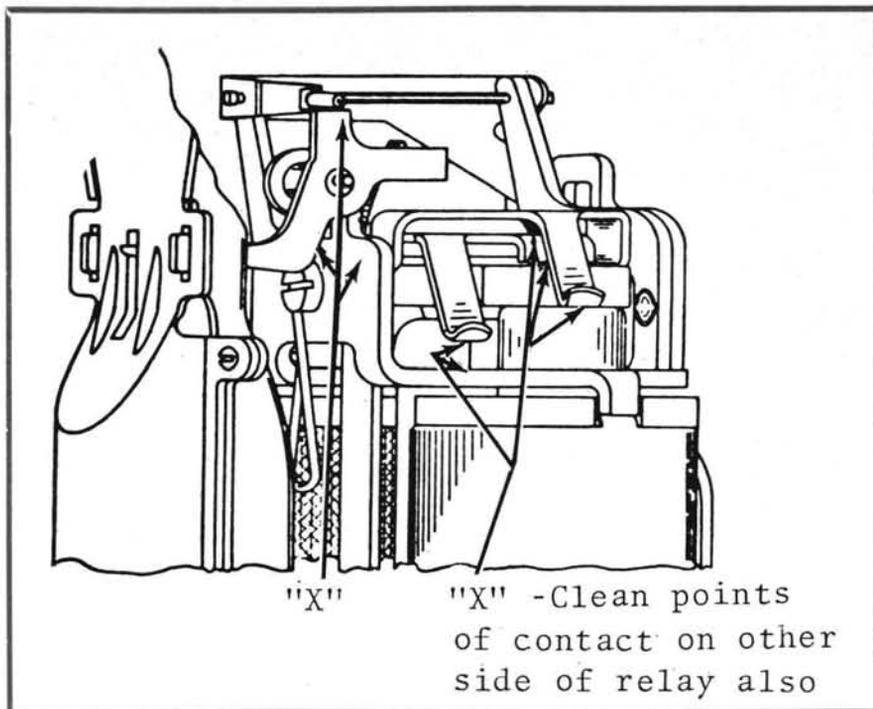
ularly to the relay armature and armature restoring arms (See Figure 4).
