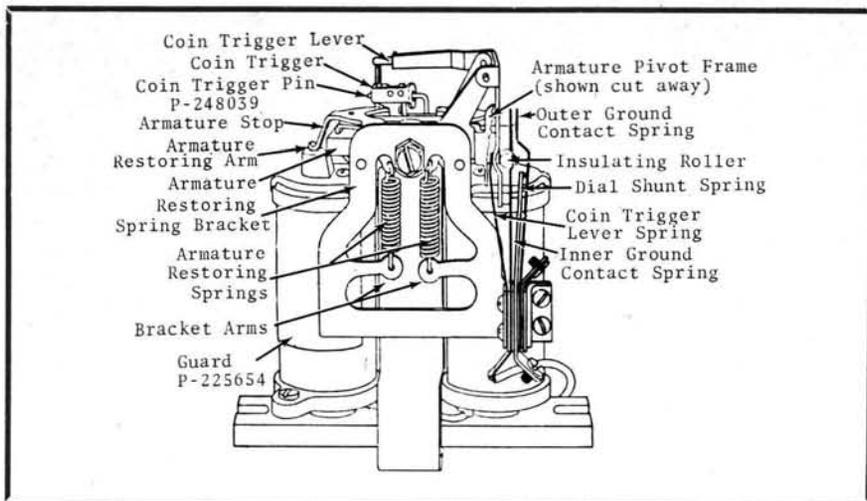
Fig. 1 Two-coil prepay coin control relay.
