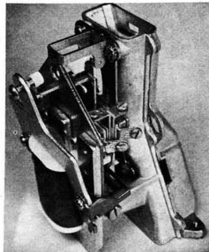
Fig. 2 Single-coil relay.
