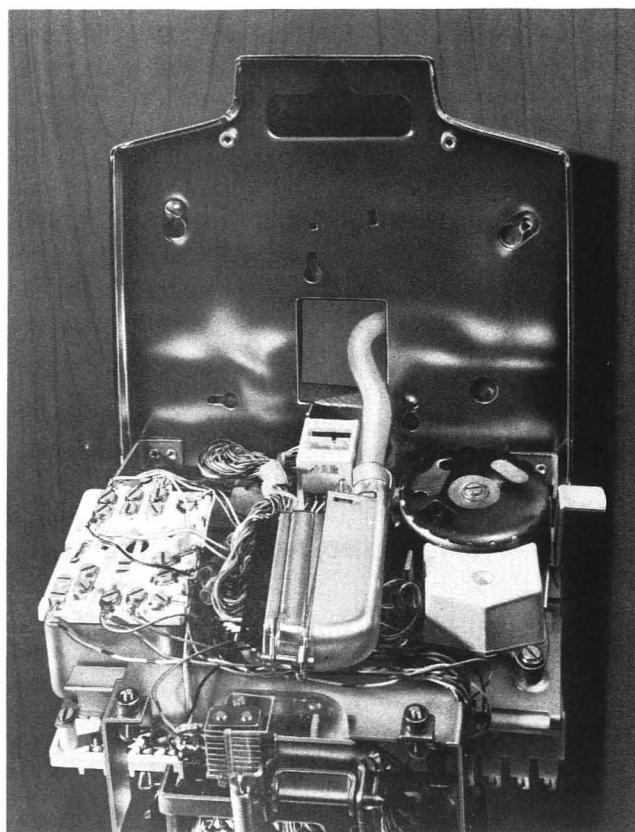
Fig. 10—Connector Cable and D-180375 Kit of Parts (Early Version)
